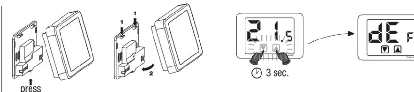
Unhook and re-hook the thermostat from the base. Press the keys for at least 3 seconds during the flashing.
